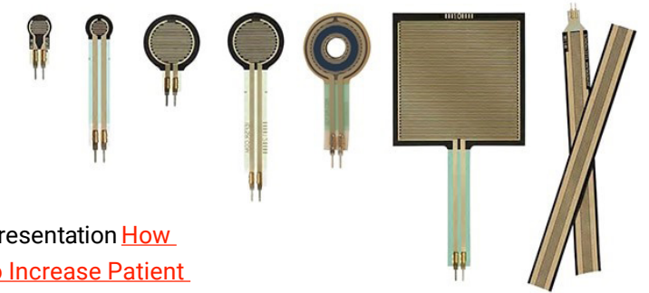
Figure 2: FSR 400-series single-zone force sensing resistors are robust polymer thick film devices that exhibit a decrease in resistance with an increase in applied force. Sensitivity is suitable for use in human-machine interfaces, medical systems, and robotics. Image source: Interlink Electronics
