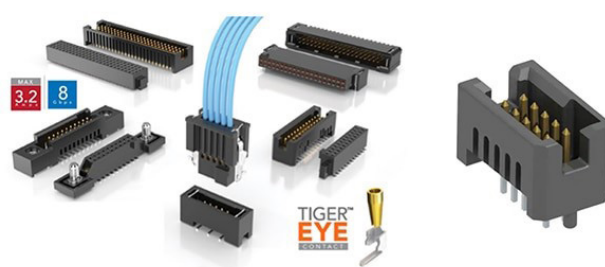
Figure 3: Tiger Eye interconnects (left) are available in a variety of formats and sizes and provide a rugged contact system rated to 10,000+ mating cycles. The TFM-105-01-S-D-A (right) is a 10-position header with 1.27mm pitch contacts.
