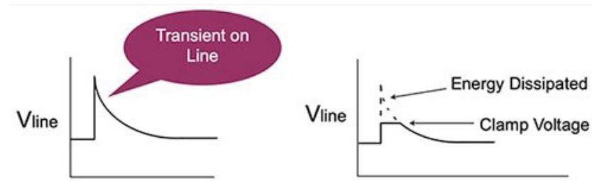
Figure 5: The abrupt switch of the MOV from high impedance to low impedance when a transient voltage occurs clamps that voltage to an acceptable level. Image source: Littelfuse, Inc.
