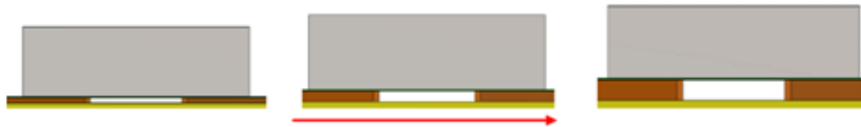
Figure 5. Increasing Top Layer PCB Copper Thickness
